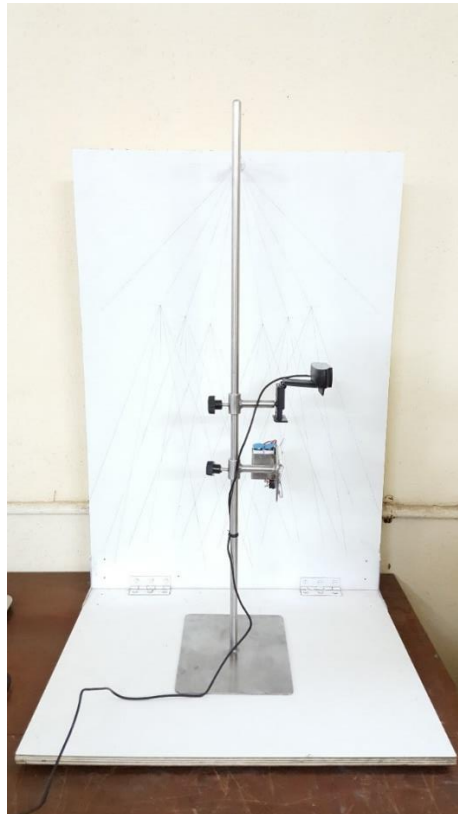
Figure 4.6: Sensor Stand with Illumination module
