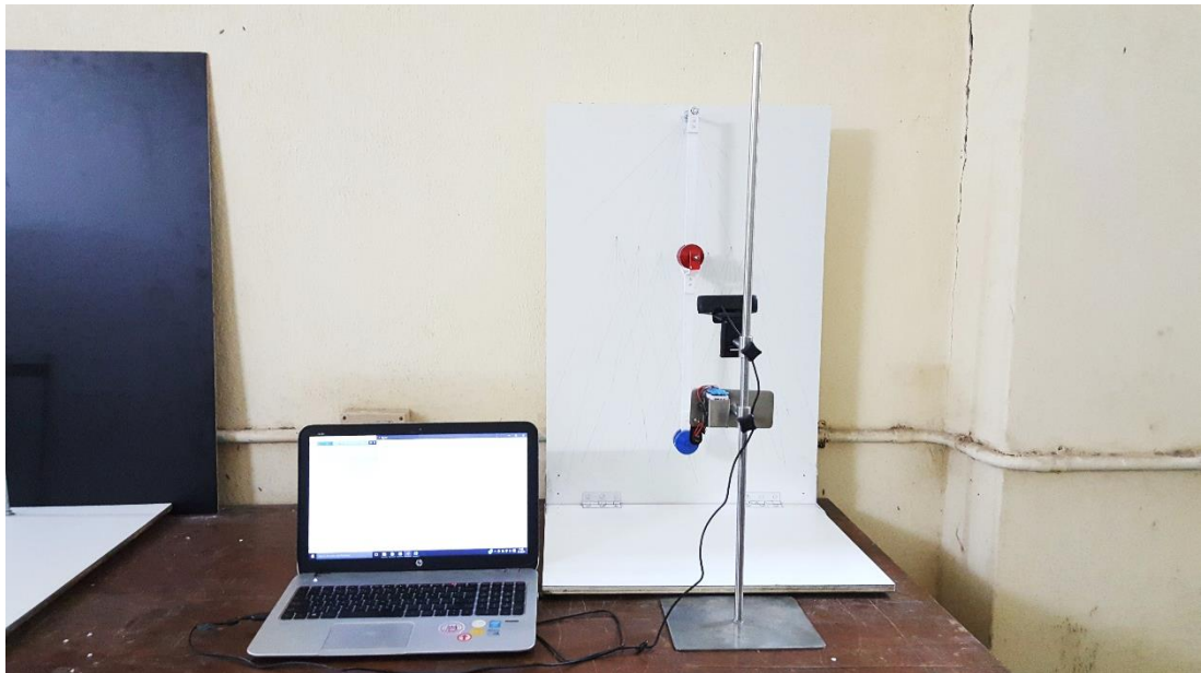
Figure 4.5: Experimental Set-up for the Study of Two DOF System
